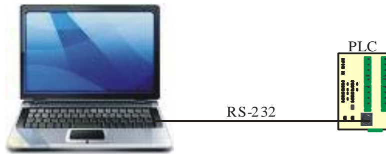
Figure (6.2): PLC RS232 connection
